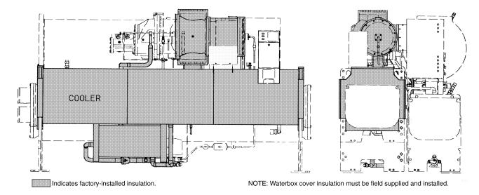
Fig. 33 — 23XL Insulation Area for Frame 4 Machines
